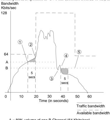
A = 80% volume of one B-Channel (64 Kbits/sec) B = 30% volume of one B-Channel (128 Kbits/sec)
